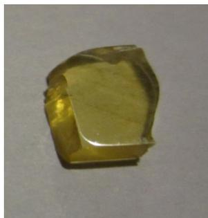
**Figura 1.** Vidrio  $\text{BTNA:Dy}^{3+}$
