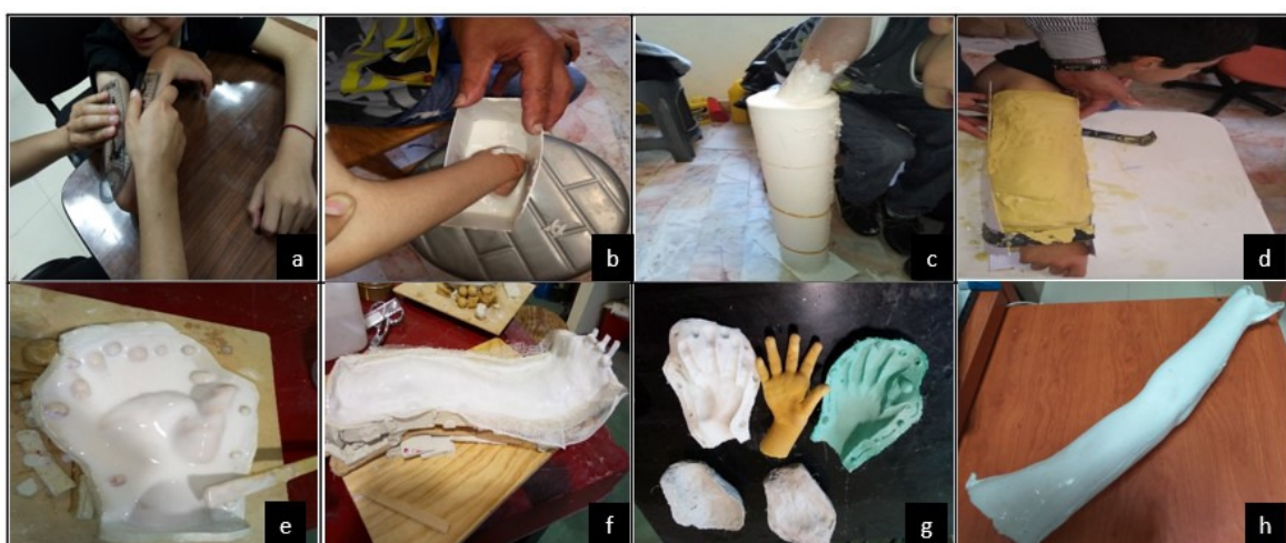
Fig. 4.3 Generation process of (a) patient upper limb characterization. (b–d) casting models. (e,f) silicon models made of (Polysil P-48™) and (g,h) dummy limbs from [2]
