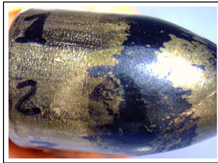
Figure 9. Deformed (experimentally) 9 mm bullet in a hexagonal barrel.
