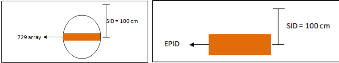
Figure 2B (left side). Phase 1, measurement geometry with the Octavius 4D system. The rotation unit and the ionization chamber array were used with a SID=100 cm. Figure 2C (right side). Phase 1, measurement geometry with portal dosimetry. The electronic portal imaging device (EPID) was placed at SID=100 cm.
