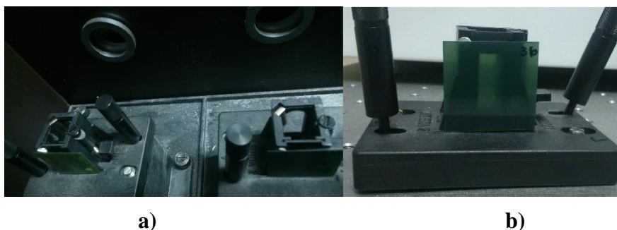
Figure 1: Spectrophotometer sample compartment. a) Photograph shows the sample holders for the non-irradiated (left holder) and the irradiated (right holder) EBT3 radiochromic films. b) Front view of the irradiated EBT3 radiochromic film mounted on the right holder.
