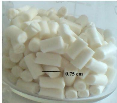
**Figure 1. Q-C Cryogels obtained by the process ISISA**
