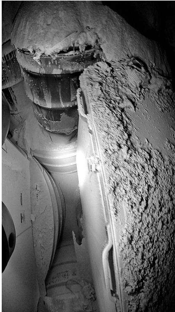
FIGURE 2.3 Damaged drum with radioactive waste inside WIPP Panel 7, Room 7, New Mexico, USA, 2014–05–15 during investigations on the cause of radioactive contamination. (DoE Photographer, damaged drum with radioactive waste inside WIPP Panel 7, Room 7, New Mexico, USA, 2014-05-15 during investigations on the cause of radioactive contamination. Retrieved June 4, 2017, from https://en.wikipedia.org/wiki/File:WIPP_DoE_2014-05-15_5_15_Image_lrg.jpg , 2014.)
