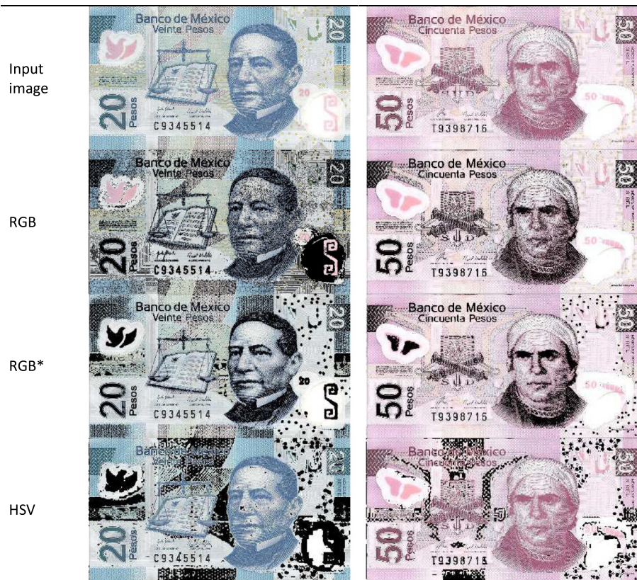
Fig. 8. Comparison between RGB and HSV color spaces for discriminative color selection applied for Mexican banknote recognition.
